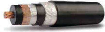
Single Core Cables, with stranded Circular copper or Aluminum conductors, XLPE insulated, aluminum wire armoured and PVC Sheath.
