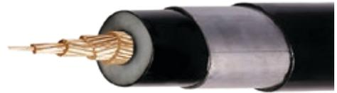
Stranded circular or segmental compacted copper conductor, semi-conducting layer as conductor screen, XLPE insulated, semi-conducting layer as non metallic insulation screen, semi conductive water blocking tape to protect the screen area from longitudinal water penetration, copper wire or tape as metallic insulation screen lead sheathed with suitable thickness to withstand the required earth fault current and HDPE sheathed with graphite coating or extruded semi-conducting layer.
