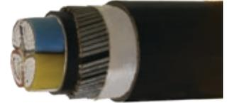
Multicore Cables, with Stranded Aluminium Conductors, PVC Insulated, Steel Wire Armoured and PVC Sheathed
